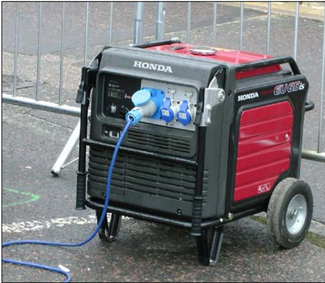
Generators should be kept dry and operated on dry surfaces.
